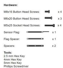
1. Use the 8 x 16 screws to fasten the base to the stage.
