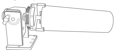
1. Position the chosen object inside the chuck jaws of the rotary (as seen above). Verify that the object is level by utilizing the included level prior to initiating the engraving process. To secure and stabilize longer or heavier objects, a jack is also included.
