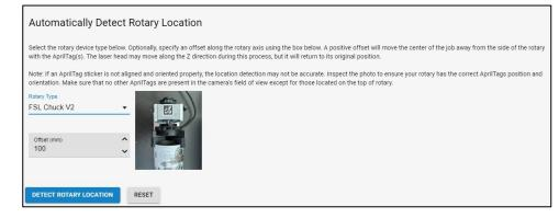
Make sure your rotary is facing the vertically and that the QR stickers are not damaged before starting.
