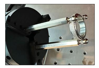
Install the rod attachment onto the machine. Position the ring onto the curvatures of the attachment. Adjust the position of the rod attachment so that the ring off-center.
