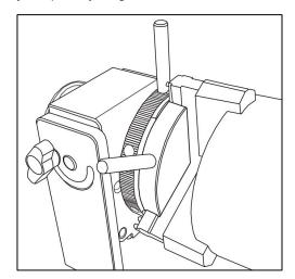
4. The dial tools are inserted into the dial holes (shown above) and then used to tighten the dial further.
