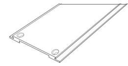
3. Grab the End Piece and slide it into the notches in the rail.
